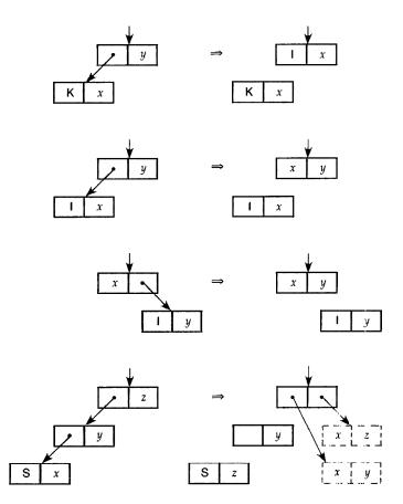
FIGURE 3. Patterns of Combinator Reduction
